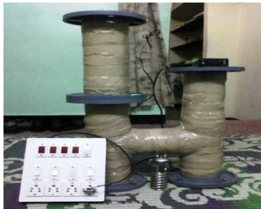
Figure 5: Test Rig for Checking Thermal Conductivity of Material
